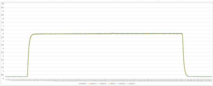
Test result: 2 hours ventilation, range drift <20ppb;
