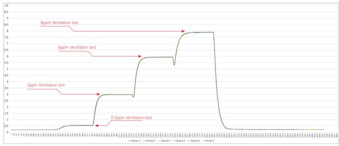
Test result: 0 ~ 10ppm linear error <± 5%;
