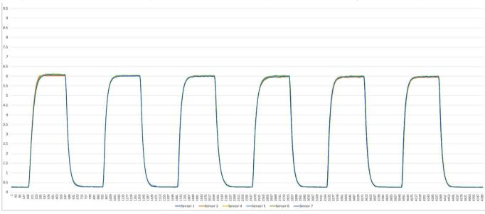
The test results show that the repeatability error range is <20ppb (10ppm  $\pm$  1% of full scale is the normal range);
