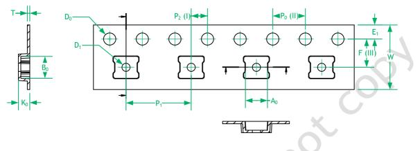
Figure 7 Drawing of the tape & reel
