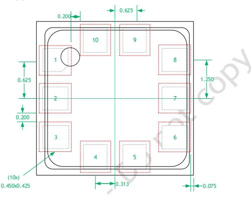
Figure 5 Recommend LGA landing pattern (Top view)
