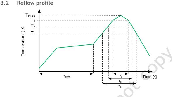
Figure 6 Solder reflow profile graph
