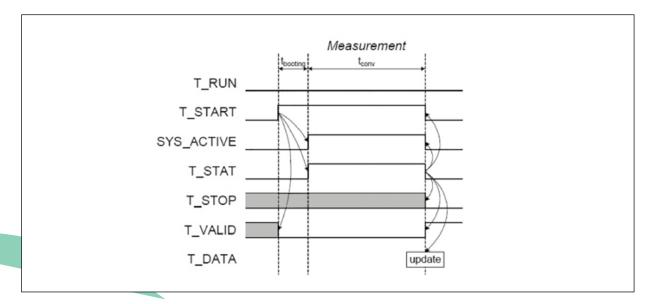
Signal T\_RUN is written low to select a single shot measurement. Note that T\_STOP is typically low (cleared by a previous measurement), but its state is ignored in a single shot measurement. T\_START is written high to start measuring: T\_VALID in T\_VAL is cleared and the device starts booting to active. Once active SYS\_ACTIVE goes high, and measurement starts (T\_STAT goes high).
