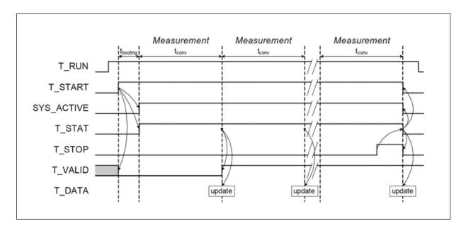
Signal T\_RUN is written high to select a continuous measurement. Note that T\_STOP is typically low (cleared by a previous measurement), and it should stay low otherwise continuous mode will stop after one measurement. T\_START is written high to start measuring: T\_VALID in T\_VAL is cleared and the device starts *booting* to *active*. Once *active* SYS\_ACTIVE goes high, and measurement starts (T\_STAT goes high).
