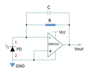
$$\begin{split} & V_{out}(V) = I_{ph}\left(A\right) \times R\left(\Omega\right) \\ & I_{ph}\left(A\right) = R_{\lambda}(A/W) \times A\left(cm^2\right) \times P\left(W/cm^2\right) \\ & \text{where A is chip area, P is incident UV power density} \\ & \text{and } R_{\lambda} \text{ is responsivity at specific wavelength.} \end{split}$$
