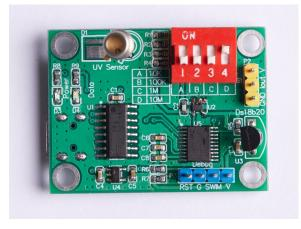
The evaluation board supports measurement range adjustment function via a dip switch. Different setting of the dip switch corresponds to different load resistance value, which determines the amplification magnitude of the signal processing circuit. A temperature sensor on board is used for embedded temperature compensation.
