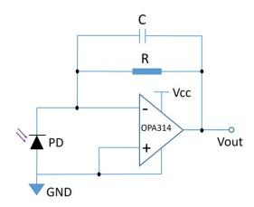
$$V_{out}(V) = I_{ph}(A) \times R(\Omega)$$
