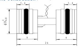
The suggested installation dimension is  $\Phi 19\,^{+0.05}_{+0.02}\,\text{mm}$
