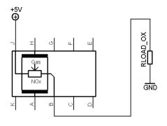
MiCS-2714 with recommended supply circuit (top view)
