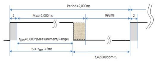
EX)  $t_H$  (High Pulse Width) calculation for 400 ppm in 2,000 ppm Range. \*Measurement<sub>(ppm)</sub> = 400 ppm = (t<sub>H</sub>-2ms)/2,000msec x Range<sub>(ppm)</sub>, \* $t_H$ = 1,000 msec \* (400 ppm / 2,000 ppm) + 2msec = 202msec (cf:  $T_L$ = Period -  $t_H$  = 2,000 ppm - 202 msec = 1,798 msec.)
