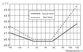
Figure 3 Typical error and maximum error of temperature
