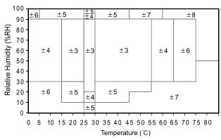
Figure 5 Maximum humidity error between 0~80 °C, unit: (% RH)
