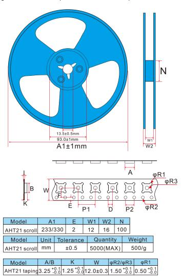
Figure 22: Package tape and sensor location diagram
