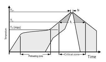
Figure 9 JEDEC Standard welding procedure diagram. Tp<= 260%, tp< 30 sec, lead-free welding.TL< 220%, tl< 150 sec,The rate of temperature rise and fall during welding shall be < 5%/ sec.
