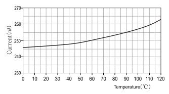
Figure 6 When VDD = 3.3V, the typical relationship between supply current and temperature (dormancy mode). Please note that there is a deviation of about  $\pm\,25\%$  with the display value.
