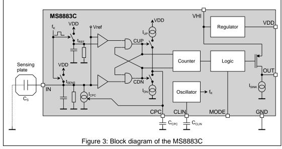
Figure 3 illustrates the functional principle of of the MS8883C
