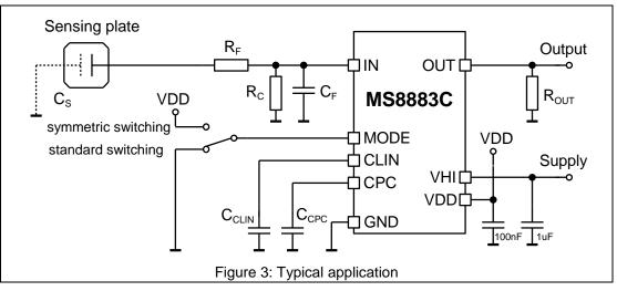
The sampling rate is determined by the capacitance  $C_{CLIN}$  on pin CLIN. The rate can be adjusted from 300Hz to 3kHz. A 1kHz rate can be defined using  $C_{CLIN} = 22pF$ . A higher sampling rate reduces the reaction time and increases the current consumption.
