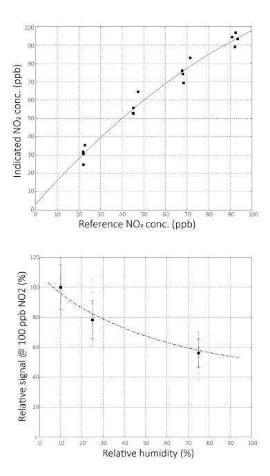
**Figure 1:** Typical sensor performance at exposure to varying concentrations of  $NO_2$ . The reference concentration is determined with an Ecotech Serinus 40 analyser. The analysis was conducted in an ambient of synthetic air at room temperature (25 °C), atmospheric pressure, and under dry conditions. The responses shown are the processed and temperature compensated signal.
