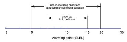
The performance assurance of methane gas detector using FSM-G-11 when alarming point is 10%LEL
