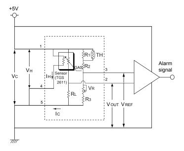
Vc: Loop voltage  $\hspace{1cm}$  lc: Loop current Vh: Heater voltage  $\hspace{1cm}$  I $_{H}$ : Heater current
